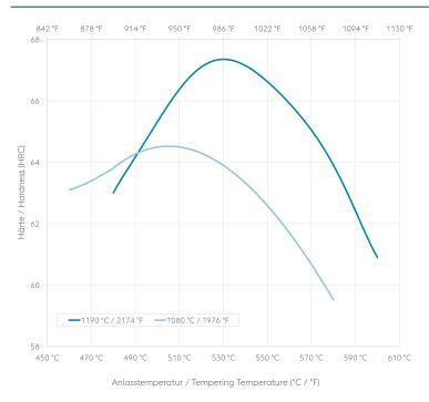
Holding time 3 x 2 hours Specimen size: square 25 mm
