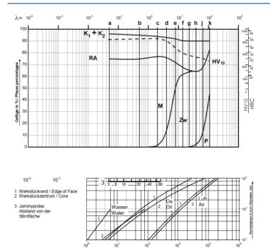
Kühlzeit von 800°C auf 500°C in Sek. Cooling time in sec. from 800°C to 500°C (1470-930°F) A....Austenite Zw....Bainite K....Carbide P....Perlite M....Martensite RA...Retained Austenite
