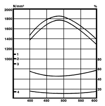
Auslagerungstemperatur (Haltedauer 3 Stunden) in  $^{\circ}$ C Ageing temperature (holding time 3 hours) in  $^{\circ}$ C
